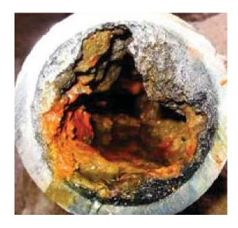
Accumulated FOG creates blockages in private sewer lines and sewer pipes, causing serious problems, including sewer back-ups into homes and businesses. FOG blockages can also lead to sewage overflows onto streets and parking lots, and interfere with sewage treatment processes at the wastewater treatment plant.
